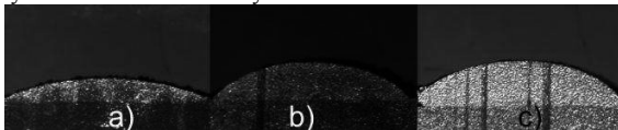
Fig. 5. Cross sections of clads, obtained with nozzles of different configurations (PMFR – 40 g/min, V \sim 20 mm/min), where: a) ordinary flat nozzle; b) nozzle with splitter and converging powder supply channels inside the nozzle body, c) nozzle with splitter and parallel powder supply channels inside the nozzle body
