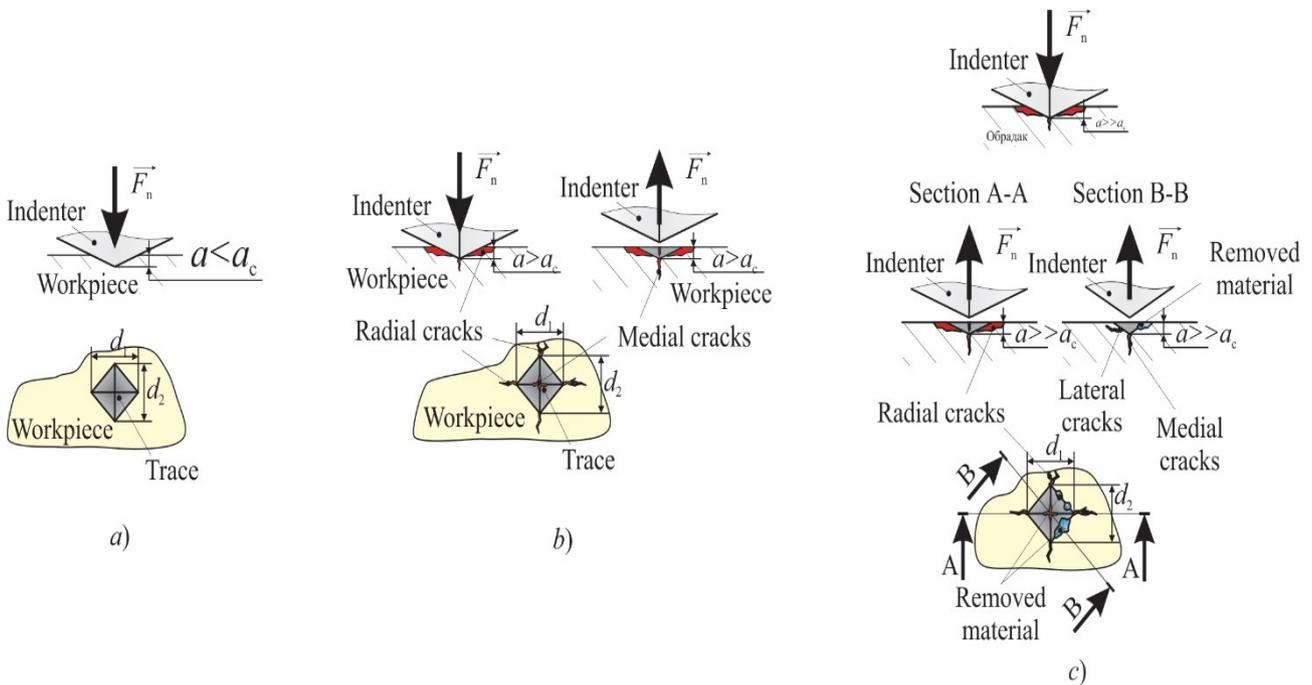
Fig. 1. Static indentation process [3]
