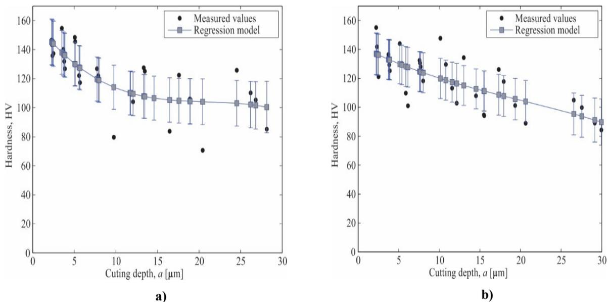
Fig. 3. Values of the hardness for a)  $T=0$  and b)  $T=15 \text{ sec}$
