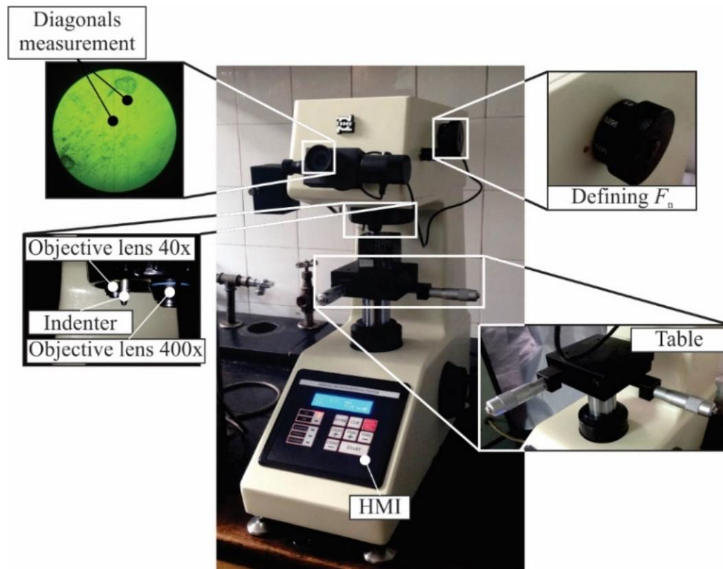
Fig. 2. Experimental setup
